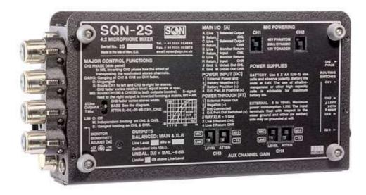
The essential information for connecting to and operating the mixer is permanently printed on the baseplate.
